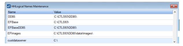
Also verify the HHDATASEND and HHDATARECEIVE lines in the HHLogical Names table and the MSDATASEND and MSDATARECEIVE lines in the MSLogical Names tables. These need to be correct prior to running downloads to mobile devices.
